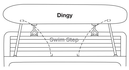
**Step 1** — Mount the brackets at a 10:00 and 2:00 o'clock position. This will provide rigidity for the dinghy. See above figure.
