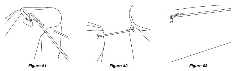
**Step 2** — Next mount the Stand-Off Cips to the dinghy and then mount the second set to the transom of the yacht. It is not recommended to put the clips on the top of the gunwhale. For inflatable boats, a rubber pad is mounted on the bow for ataching the Stand-Off clip. The Stand-off Clip can be mounted into wood or fiberglass transoms for the stern hook-up. See figures #1 and #2.
