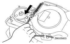
Remove the starter/flywheel cover after removing the bolt(s).
