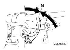
Place the tilt lock lever in the release/up position.
