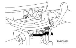
3. Hold the handgrips and steering brackets as shown in the illustration and lift up the outboard motor using two people.
