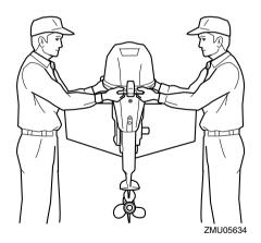
When transporting or storing the outboard motor while removed from a boat, keep the outboard motor in the attitude shown.
