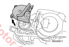
Remove the electrical system cover by removing its screw(s).
