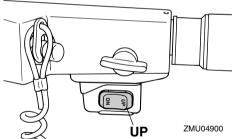
B. Push the tilt support knob into the clamp bracket to support the engine. WARNING! After tilting the outboard motor, be sure to support it with the tilt support knob or tilt support lever. Otherwise the outboard motor could fall back down suddenly if oil in the power trim and tilt unit or in the power tilt unit loses pressure. [EVMIOD263] NOTICE: Do not use the tilt support
