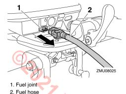
3. Disconnect the fuel hose from the fuel joint on the fuel tank.
