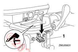
1. Tilt lock lever (Release / tilt-up)
