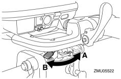
If the resistance does not increase even when the lever is turned to the port side "A", make sure that the nut is tightened to the specified torque.
