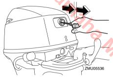
After the engine starts, slowly return the manual starter handle to its original position before releasing it.
