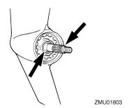
Check the propeller shaft oil seal for damage.
