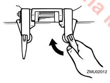
If the restraint cable attachment is equipped on your engine, a restraint cable or chain should be used. Attach one end to the restraint cable attachment and the other to a secure mounting point on the boat. Otherwise the engine could be completely lost if it accidentally falls off the transom.
