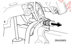
Push the power tilt switch "DN" (down) to lower the outboard motor to the desired position.
