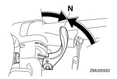
Slightly tilt the outboard motor up to the desired position using the power tilt switch. WARNING! Using the power tilt switch on the bottom cowling while the boat is moving or engine is on could increase the risk of falling overboard and could distract the operator, increasing the risk of collision with another boat or an obstacle.
