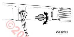
When constant speed is desired, tighten the adjuster to maintain the desired throttle setting.
