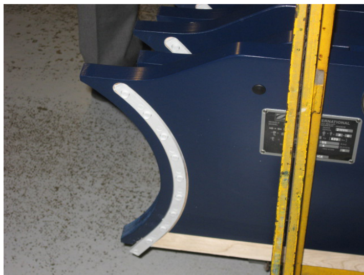
Rivet rails attached to transom prior to cuff welding
