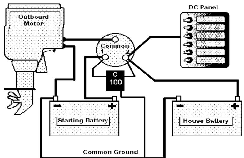
or both can be selected in an emergency. In all cases, both batteries are being charged when the engine is running. **WARNING:** If you use this circuit, turning the switch to "OFF" while the engine is running may damage your alternator.
