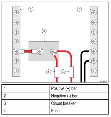
Where possible, connect individual items of equipment to individual circuit breakers. Where this is not possible, use individual in-line fuses to provide the necessary protection.
