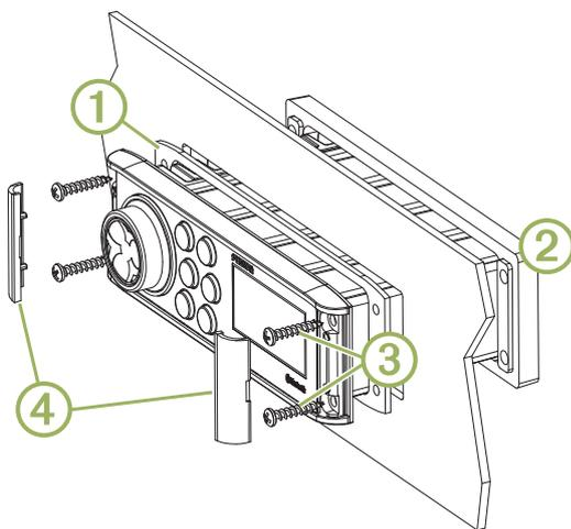
4 Place the mounting bracket ② behind the mounting surface.
