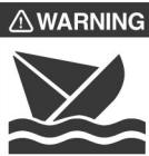
**Flood hazard.** Before performing any service, close all waste system seacock. Failure to do so can result in flooding which can cause loss of property and life.
