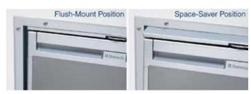
CRX refrigerators in black and silver finish come standard with a flange to match the door panel color. In the flush-mount position, the flange provides a pleasing cosmetic appearance and eliminates a protruding handle or locks. In the space-saver position, the flange is set about an inch back for installations where cabinet depth is limited. The flange must be ordered separately for stainless-steel CRX models.
