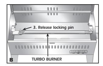
**3.** To remove burner pull locking pin.
