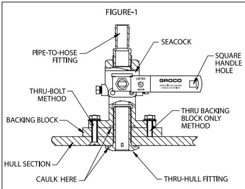
**Reversing Handle Rotation:** GROCO BV seacocks include the patented user-selectable handle rotation feature. If seacock location does not allow unobstructed handle operation, you may change the rotation direction by relocating the set-screw (Exploded View Item-17). The set-screw may be removed altogether if 180-degree handle rotation is desired.
