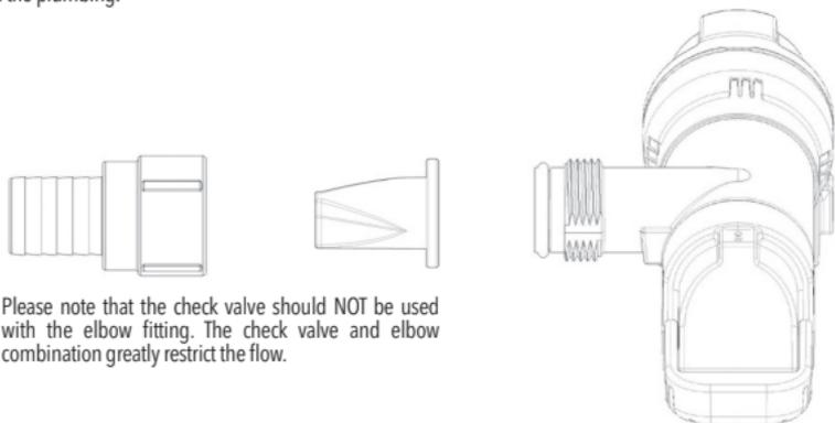
Please note that the check valve should NOT be used with the elbow fitting. The check valve and elbow combination greatly restrict the flow.
