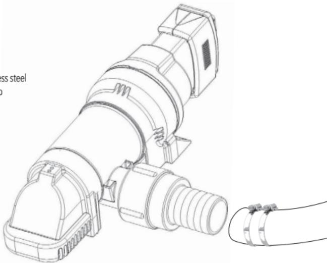
During the winterization of a vessel, it's recommended that you remove the check valve (if equipped) and drain any residual water from the plumbing.
