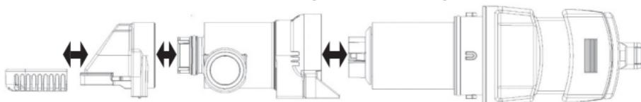
Best practice: Periodically clean the sensor housing with a mild detergent to remove any build-up that may interfere with the proper operation of the bilge pump. If the sensor accumulates excessive build-up, the pump will enter the timer mode to protect the pump and the vessels batteries. Once the debris is removed, the pump will return to level sense mode.
