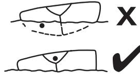
Install overboard discharge well above both static and heeled waterlines.
