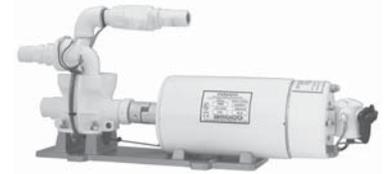
To enable NOFLO™ remove the jumper wire. During normal operation NOFLO™ will sense the absence of water and turn the pump off after 30-seconds of continuous dry running. If your Paragon pump ever shuts off when you know that water is present and the pump has not exceeded 10-minutes of continuous running, reconnect the jumper wire to disable NOFLO™.
