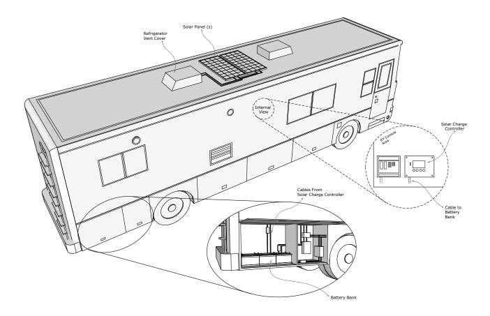
FIGURE 2-A: TYPICAL RV INSTALLATION
