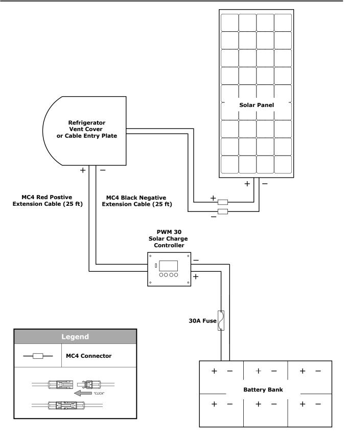
FIGURE 2-B: FLEX 100 WIRING DIAGRAM
