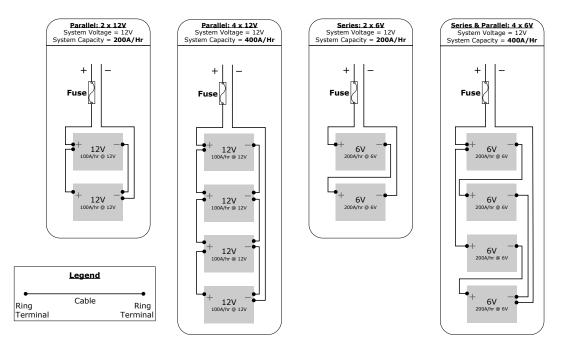
FIGURE 4-J: TYPICAL BATTERY BANK CONFIGURATIONS
