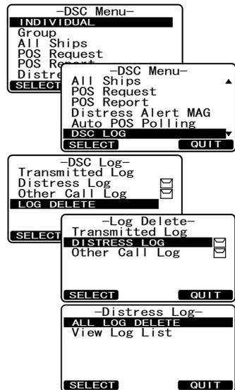
2) If you want to delete one of the logged stations, select the "VIEW LOG LIST" with the **CH** knob, then press the **SELECT** soft key. Rotate the **CH** knob to select the station (name or MMSI number) to be deleted, then press the **DELETE** soft key.
