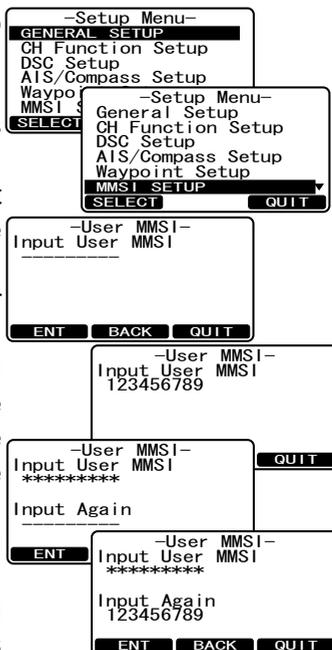
8. After the second number has been input, press and hold the **CH** knob to store the MMSI.
