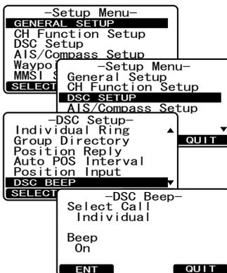
To re-enable the ringer tone, repeat the above procedure, rotating the **CH** knob to select “On” in step 6 above.
