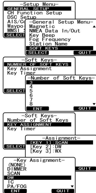
9. Press the **QUIT** key, then rotate the **CH** knob to select “KEY TIMER” (selects how long the soft key icon will be shown on the display after a soft key is pressed, default is 5 seconds). Then, press the **SELECT** soft key.
