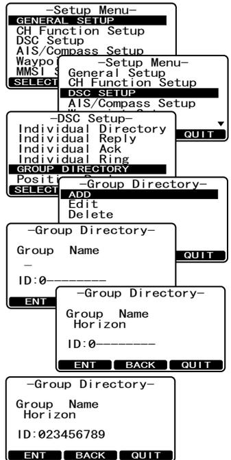
If a mistake was made entering in the name repeat pressing the **BACK** soft key until the wrong character is selected, then rotate the **CH** knob to correct the entry.
