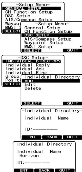
If a mistake was made entering in the name repeat pressing the **BACK** soft key until the wrong character is selected, then rotate the **CH** knob to correct the entry.
