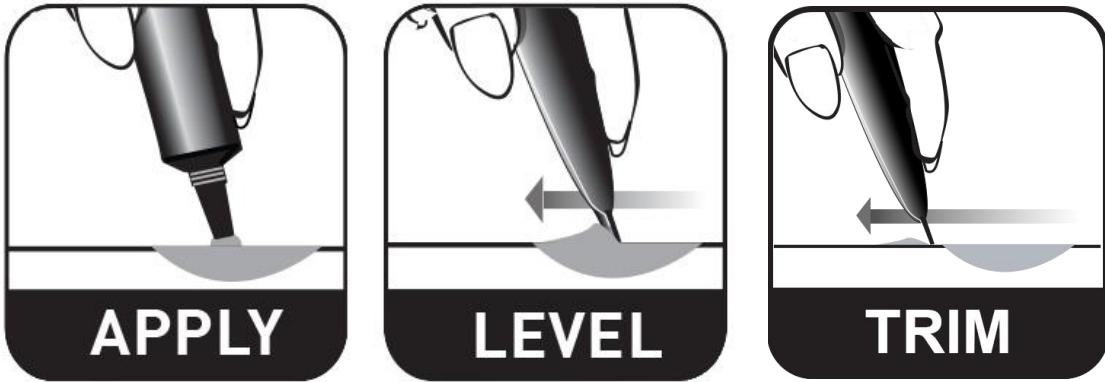
**Note:** When using Hairline Fix as a glossy top coat to a 9 Second Chip Fix Repair, follow Step 3 – Apply and level
