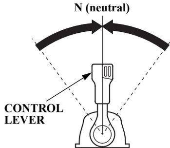
1. Move the throttle grip to the slowest speed and the gearshift lever or control lever to the N (neutral) position.
