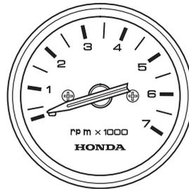
The tachometer shows engine speed in revolutions per minute.
