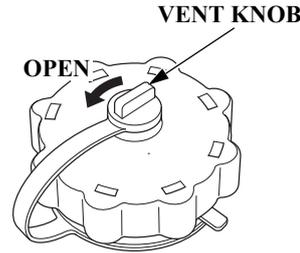
2. Turn the fuel filler cap counterclockwise so that it touches the pressure relief tab.
