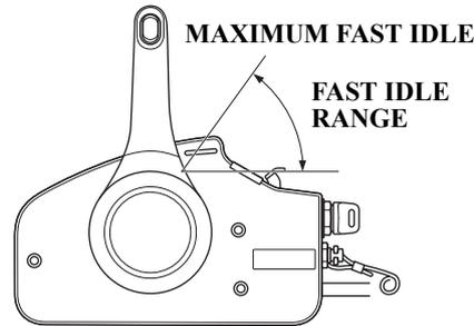
6. Before getting underway, allow the engine to warm-up sufficiently to ensure good performance.
