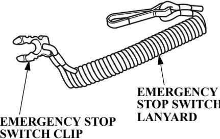
The emergency stop switch clip must be inserted in the emergency stop switch in order for the engine to start and run. The emergency stop switch lanyard must be attached securely to the operator or to the operator’s PFD (Personal Flotation Device).
