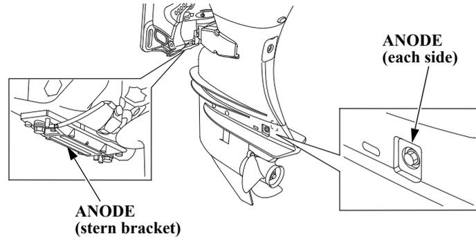
The anodes are located on each side of the gear case and on the stern bracket. They are made of a sacrificial material that helps to protect the outboard motor from corrosion.
