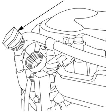
4. If the oil level is low, remove the oil filler cap, and add oil to reach the upper limit mark shown on the dipstick. Use the oil recommended on p. 101.
