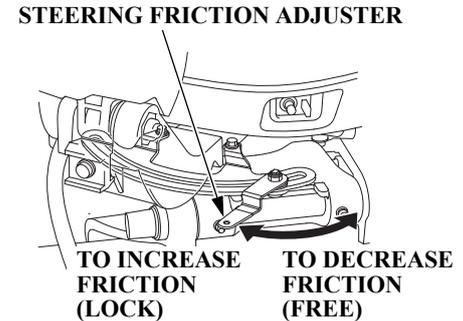
The steering friction adjuster adjusts steering resistance.
