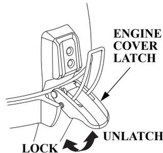
The engine cover latches fasten the engine cover to the outboard motor.
