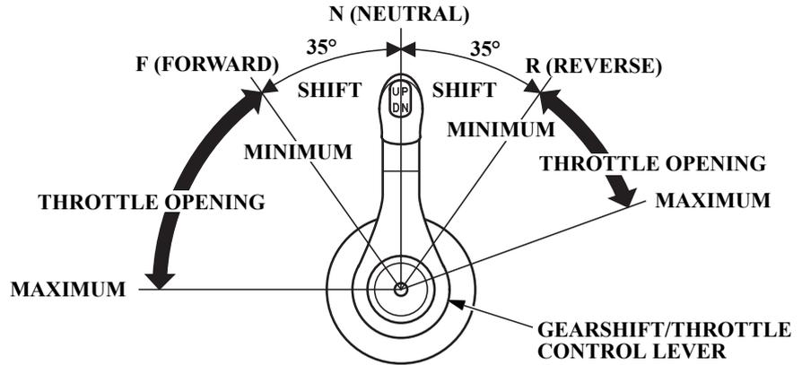
Moving the control lever 35° from N (neutral) selects the gear, and further movement increases engine speed.
