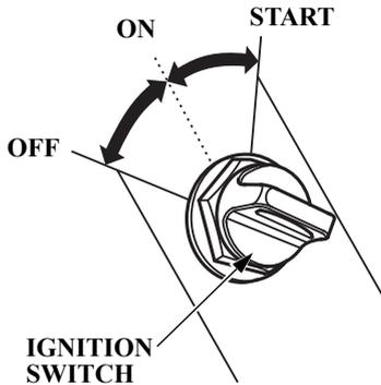
The ignition switch controls the ignition system and the starter motor.
