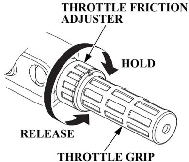
The throttle friction adjuster adjusts resistance to throttle grip rotation.
