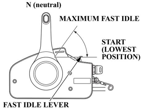
Use the fast idle lever to accelerate engine warm-up after starting the engine. Do not use the fast idle lever when starting the engine.
