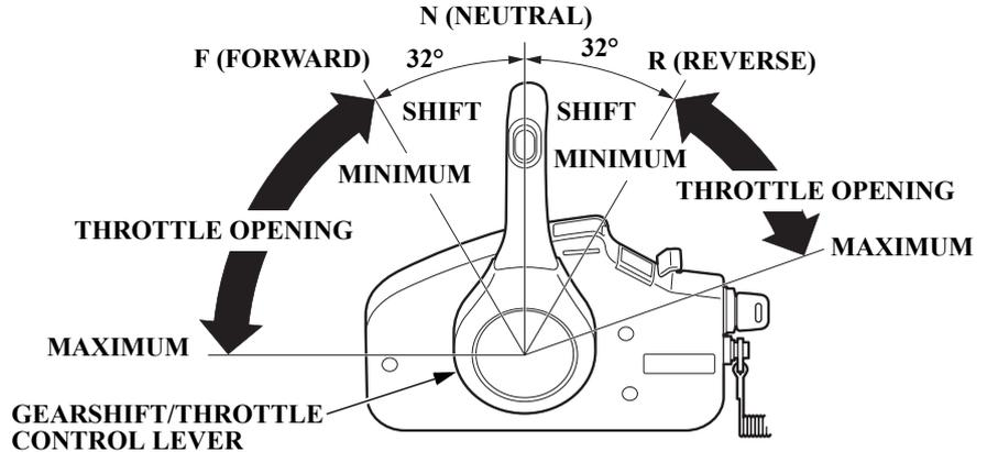
Moving the control lever 32° from N (neutral) selects the gear, and further movement increases engine speed.
