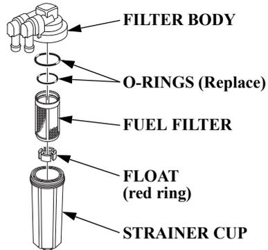
6. Unscrew the strainer cup from the filter body.
