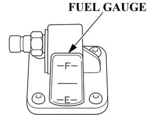
A fuel gauge is built into the fuel tank connector of the portable fuel tank.
