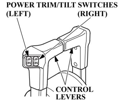
The power trim/tilt switch is located on the control lever. It is a rocker switch with UP and DN (down) positions for changing the angle of the outboard motor.
