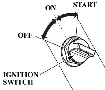
The ignition switch controls the ignition system and the starter motor.
