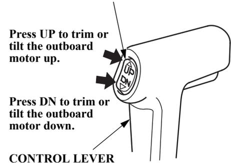
Press UP to trim or tilt the outboard motor up.
