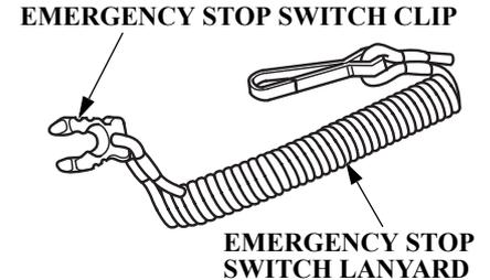
The emergency stop switch clip must be inserted in the emergency stop switch in order for the engine to start and run. The emergency stop switch lanyard must be attached securely to the operator or to the operator's PFD (Personal Flotation Device).
