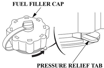
3. Press down the pressure relief tab, and then turn the fuel filler cap 1/4 turn counterclockwise. Release the pressure relief tab. Wait to relieve pressure.
