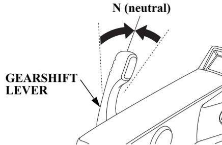
2. Check the position of the gearshift lever. It must be in the N (neutral) position for starting.
