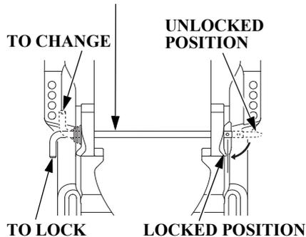
The transom angle adjusting rod limits the tilt angle of the outboard motor when fully lowered.
