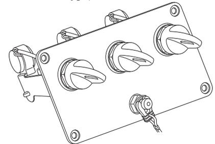
For the control panel without indicators type, use it along with the NMEA2000-compatible device.
