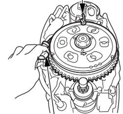
**ARROW STARTER MOTOR**      **EMERGENCY STARTER ROPE**
