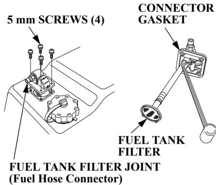
1. Remove the four 5 mm screws using a flat screwdriver, then remove the fuel hose connector and fuel tank filter from the tank.
