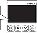
When the alert triggers, the overheat indicator comes on and the buzzer sounds a steady tone as the engine speed is reduced to 1,800 rpm. If the condition persists for another 20 seconds, the engine shuts off. Refer to *TAKING CARE OF UNEXPECTED PROBLEMS*, on p. 130.
