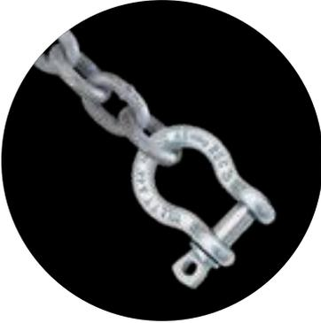
Heavy gauge chain is attached to the anchor with an appropriately sized galvanized shackle. This length of chain should be equal to 1.5 times the maximum depth of the water — accounting for extreme high tides. A swivel shackle is used to attach lighter chain to the heavy chain. This lighter chain should be equal to the maximum depth of the water, again accounting for extreme high tides.
