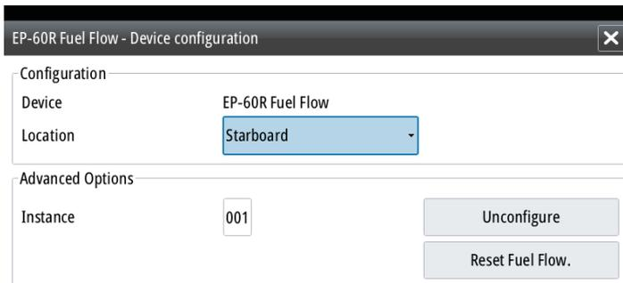
'Unconfigure' is for defaulting the device clearing all user settings, and 'Reset Fuel Flow' will restore only the 'Fuel K-Value' setting, if set in 'Calibrate'. Only Navico devices can be reset.
