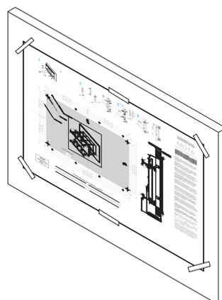
Check the template for scaling accuracy, using a tape measure or ruler against the ruler printed on the template.
