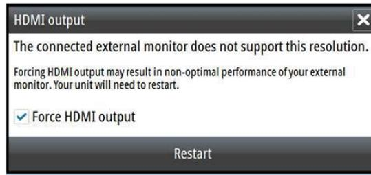
Alternatively, 'Force HDMI output' may be selected in Settings/Advanced/Features. The unit will need to restart to apply the change.
