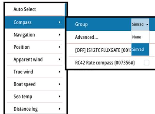
Devices with the Group set to None can be set to use different sources to those of the rest of the network devices.
