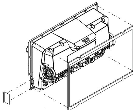
Fit the small self adhesive decal to right side of unit, covering rubber tab of SD card reader gasket. Then attach self adhesive foam gasket to rear of display.
