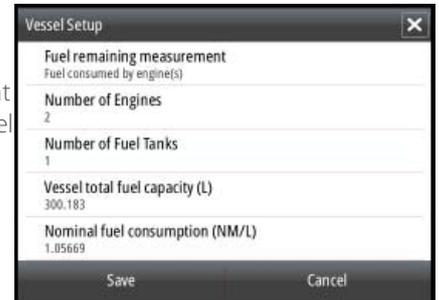
→ **Note:** Fuel remaining measurement taken from level sensors while underway may be suffer inaccurate readings due to vessel movement.
