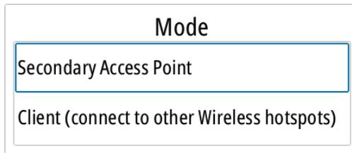
When viewing this menu for a WIFI-1 set to 'Access Point' mode, it's also possible to switch between 'Primary' and 'Secondary' access point modes so two WIFI-1 devices can exist on the network at the same time.
