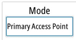
Only one WIFI-1 may operate as 'Primary', which determines that the device is acting as DHCP server. Only one DHCP server may exist on a network at a time.
