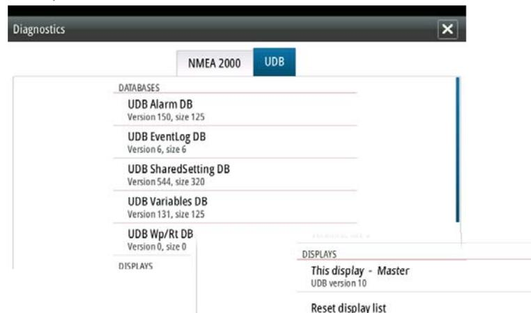
The 'Reset Display List' can be used to refresh the list of connected displays and their UDB version.
