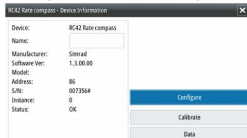
All devices allow allocation of an instance number via the **Configure** option. Set unique instance numbers on any identical devices on the network. The **Data** option shows all data being output by the device. Some devices will show additional option(s) specific to the device - the RC42 illustrated above has a **Calibration** option, to allow easy setup of this device which does not have it's own user interface.
