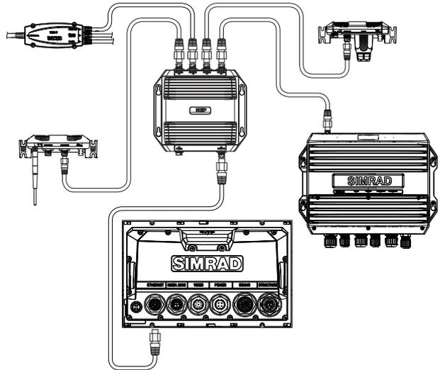
→ **Note:** some ethernet devices are equipped with two or more ethernet ports, which allow connection of additional devices, and may eliminate the need for an extra NEP-2.
