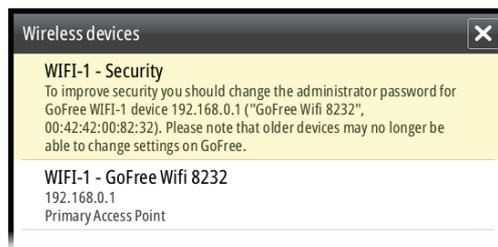
Selecting a device will provide additional details and settings specific to the selected wireless device. Displayed content depends on whether wireless is set to access point or client mode.
