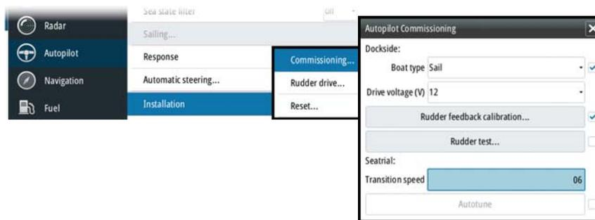
When the autopilot computer is delivered from factory AND ANY TIME AFTER AN AUTOPILOT RESET HAS BEEN PERFORMED, you will have to run a complete setup again.
