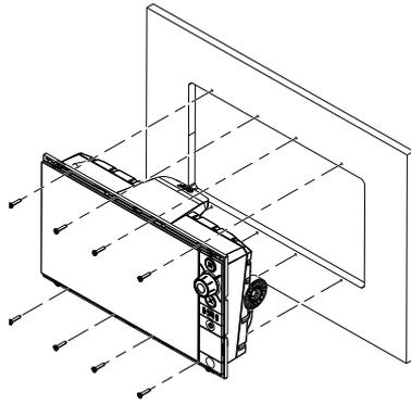
Check the fit of the display, and file away remaining obstructions. Secure the display with the supplied screws. Once screws are fully tightened, ensure there is complete contact with the mounting surface. If machine screws are required, use only M2.5 (3/32") size with a head diameter no greater than 5.6mm (7/32").
