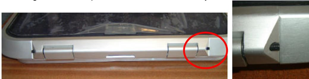
5. Clamp a pair of mole grips on to the part of the hinge pin which is sticking out. Withdraw the hinge pin
