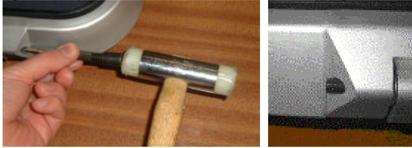
2. Close the lid without dogging the handle this minimises the load on the hinge pin. A small length of the black hinge pin should now be visible sticking out of the back of the lid where the hinge tapers away to the upper frame.
