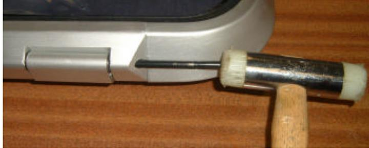
2. Use punch to push pin 2mm into hole
