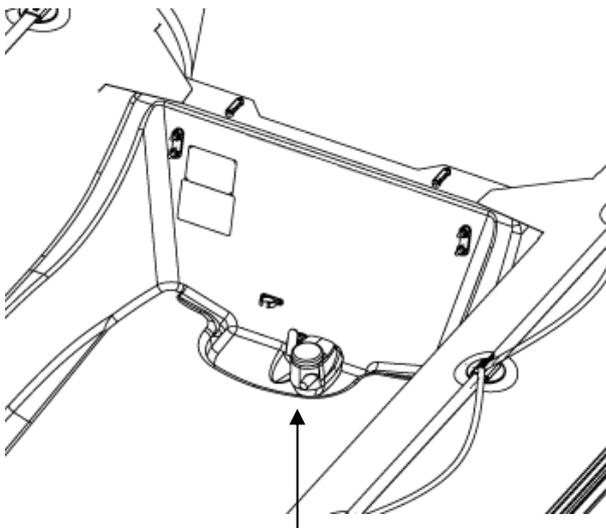
Bilge pump placed at the bottom of the aft well DB420
