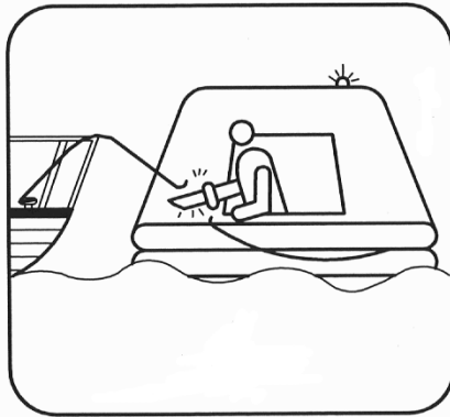
FIGURE 7 CUTTING PAINTERLINE WITH RAFT KNIFE
