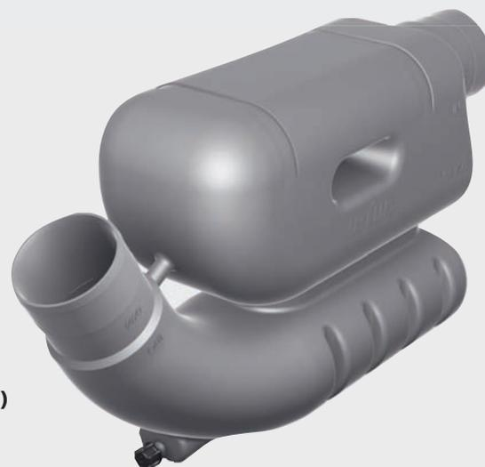
Hose connection Ø 60 mm (2<sup>6</sup>/<sub>16</sub>" ), 76 mm (3") or 90 mm (3<sup>9</sup>/<sub>16</sub>" ). With check valve and the inlet/outlet stubs will rotate through 360 degrees. Two securing straps are standard supply.
