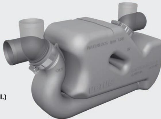
These waterlocks are designed for long relatively straight exhaust runs, for example in sailing boats. They have fixed (non-rotating) inlet and outlet connections and are available for Ø 60 mm (2<sup>6</sup>/<sub>16</sub>" ), 75 mm (2<sup>15</sup>/<sub>16</sub>" ) or 90 mm (3<sup>9</sup>/<sub>16</sub>" ) internal diameter exhaust hose. Two securing straps are standard supply.
